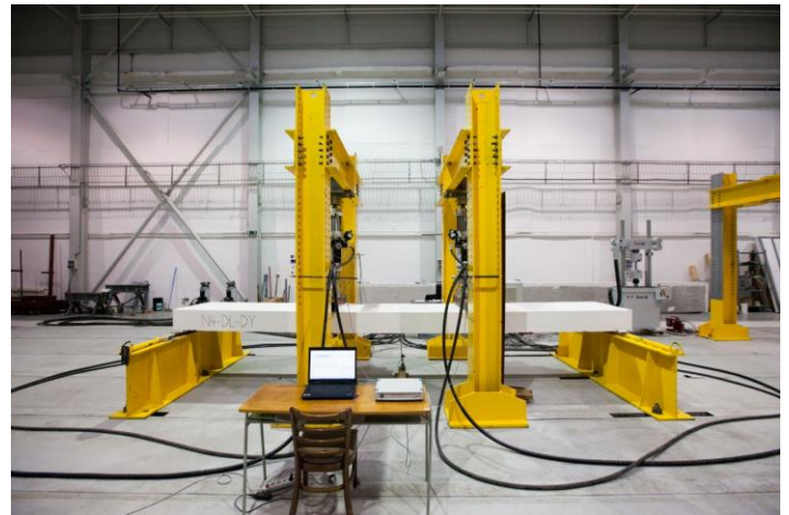
Figure 2. Static loading scheme.
